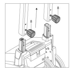
If the knobs for height adjustment [7] and the lower knobs [8] have been completely removed from the handlebar, they must not be interchanged when they are screwed back into the handlebar. The knobs for height adjustment [7] have a long thread (diagram A); the lower knobs [8] have a short thread (diagram B).
