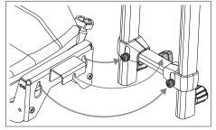
• Place the backrest [19] against the height adjustment tubes and push the backrest towards the tubes until the backrest brackets engage with the tubes.
