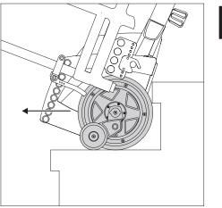
If you want to stop the stair climber while climbing a step, do not continue pressing the drive switch [4]. Alternatively, while the drive switch [4] is actuated, you can press the emergency stop switch [2]. The stair climber will also come to an immediate stop. For details of how to put the stair climber back into operation after pressing the emergency stop switch [2]: see chapter 2.7.3. Press the drive switch [4] in the correct direction.
