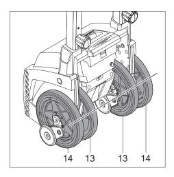
**2.8.1 Aligning the wheels manually (putting them in the wheel starting position)** In several chapters of this operating manual, you are made aware of the correct alignment of the inner [13] and outer [14] drive wheels. All four wheels must be in line with each other (see diagram), i.e. in the wheel starting position. This also ensures that these four wheels are in correct contact with the ground. You can reach this important setting by doing the following:
