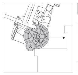
If you want to stop the stair climber while climbing a step, do not continue pressing the drive switch [4]. Alternatively, while the drive switch [4] is actuated, you can press the emergency stop switch [2]. In this case, the stair climber also stops immediately. How to put the stair climber back into operation after pressing the emergency stop switch [2]: see chapter 2.7.3. Press the drive switch [4] in the correct direction.
