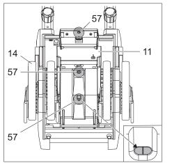
Carefully clean the three glass sensor covers [57] at the bottom of the drive housing of the stair climber if they are dirty: Wipe the glass sensor covers [57] with a dry or damp (not wet!) Wipe with a cloth or a dry or damp (not wet!) plastic-free cotton swab. If the contamination is persistent: Soak the dirt before wiping by placing a damp (not wet!) cloth or damp (not wet!) plastic-free cotton buds on the glass sensor covers for a while.
